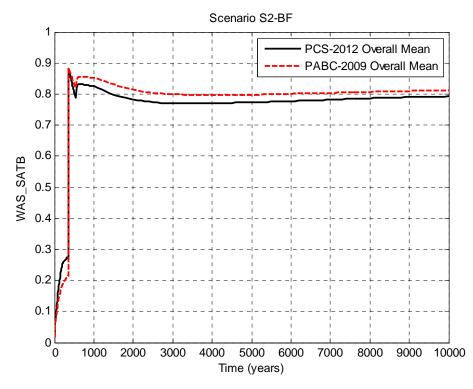
Figure 5-12: Overall Means of Waste Panel Brine Saturation, Scenario S2-BF.
