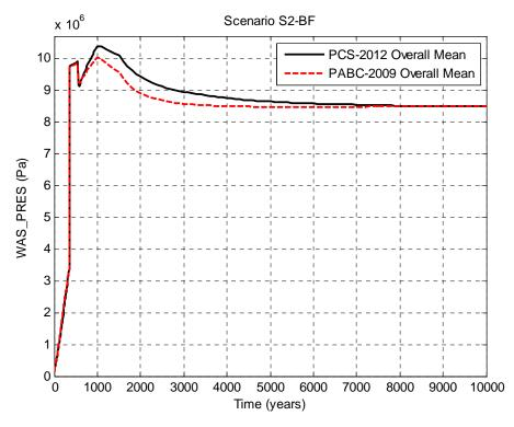
Figure 5-10: Overall Means of Waste Panel Pressure, Scenario S2-BF.
