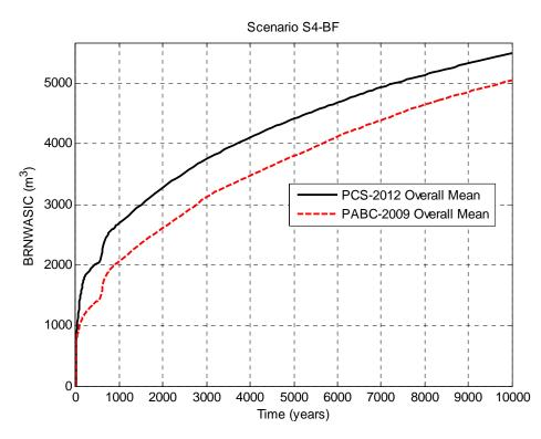
Figure 5-18: Overall Means of Cumulative Brine Inflow to the Waste Panel, Scenario S4-BF.
