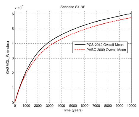
Figure 5-6: Overall Means of Waste Panel Gas Generation (in moles), Scenario S1-BF.
