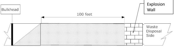
(b) Panel closure with 100 feet (30.5m) of ROM salt between a ventilation bulkhead & explosion wall
