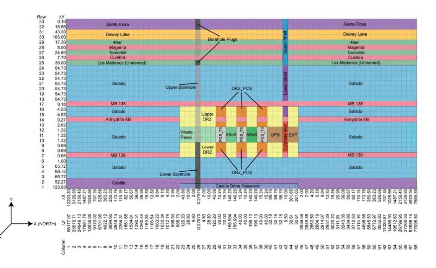
Figure 5-2: PCS-2012 BRAGFLO Grid and Material Map for an E1 Intrusion ( $\Delta x$ ,  $\Delta y$ , and  $\Delta z$  dimensions in meters).
