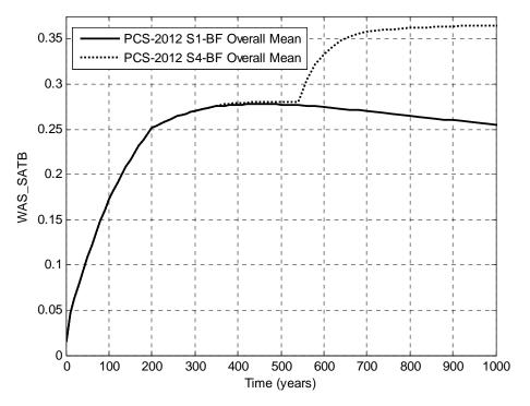
Figure 5-19: Overall Means of Waste Panel Brine Saturation, Scenarios S1-BF and S4-BF for Years 0 to 1,000.
