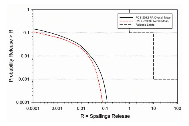
Figure 5-24: PCS-2012 PA and PABC-2009 Overall Mean CCDFs for Normalized Spallings Releases
