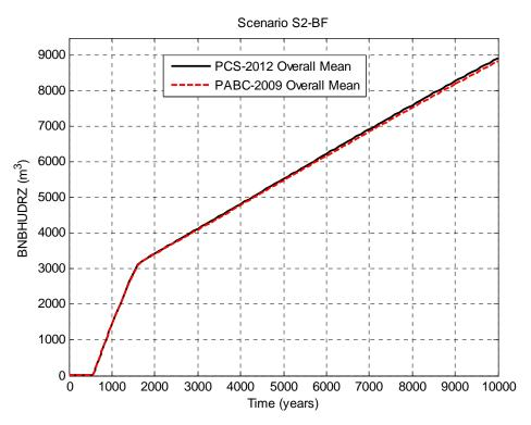
Figure 5-14: Overall Means of Brine Flow up the Borehole, Scenario S2-BF.
