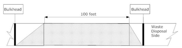
(a) Panel closure with 100 feet (30.5m) of ROM salt between two ventilation bulkheads
