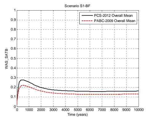
Figure 5-5: Overall Means of Waste Panel Brine Saturation, Scenario S1-BF.
