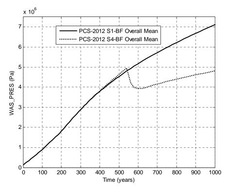
Figure 5-15: Overall Means of Waste Panel Pressure, Scenarios S1-BF and S4-BF for Years 0 to 1,000.
