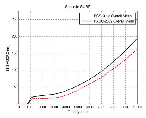
Figure 5-22: Overall Means of Brine Flow up the Borehole, Scenario S4-BF.
