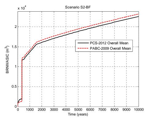
Figure 5-11: Overall Means of Cumulative Brine Inflow to the Waste Panel, Scenario S2-BF.
