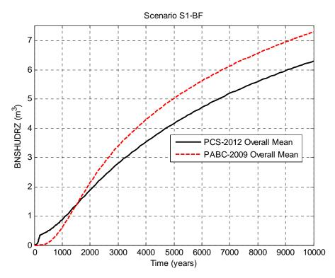
Figure 5-9: Overall Means of Brine Flow up the Shaft, Scenario S1-BF.
