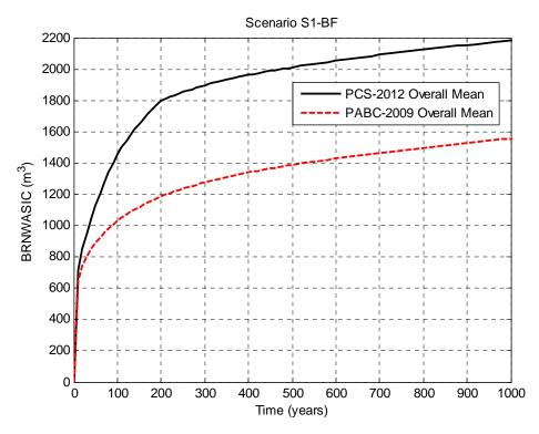
Figure 5-4: Overall Means of Cumulative Brine Inflow to the Waste Panel, Scenario S1-BF and Years 0 to 1,000.
