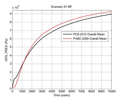
Figure 5-8: Overall Means of Pressure in the Operations Region, Scenario S1-BF.
