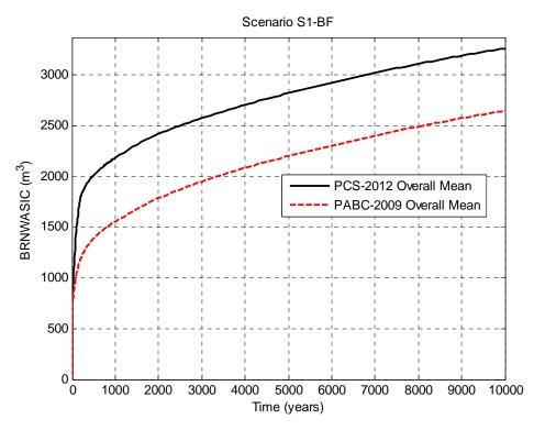
Figure 5-3: Overall Means of Cumulative Brine Inflow to the Waste Panel, Scenario S1-BF.
